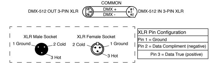
**Special Note:** Line Termination. When longer runs of cable are used, you may need to use a terminator on the last unit to avoid erratic behavior. A terminator is a 110-120 ohm 1/4 watt resistor which is connected between pins 2 and 3 of a male XLR connector (DATA + and DATA -). This unit is inserted in the female XLR connector of the last unit in your daisy chain to terminate the line. Using a cable terminator (ADJ part number Z-DMX/T) will decrease the possibilities of erratic behavior.
